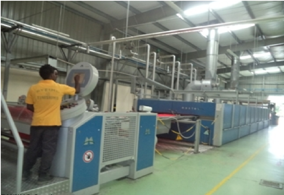
DYEING Section of the dyeing process in a textile factory. The dyeing process is 100% automated using the German companies (Germany), Tensionless dryer, Steiner & Com
