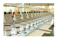
Our embroidery machine made of Barudan and Tajima with a total of *42 heads* adds value to our products. Our computeriesd automated embodiery machines enable us on providing highly precise smaller letter designs, excellent trimming system with stable performance.
